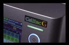
Celltac G status indicator is located in the front panel and clearly illustrates different operating status of the analyzer. For example, the operator can quickly recognize the need for reagent replacement by just looking at the status indicator turning red.
